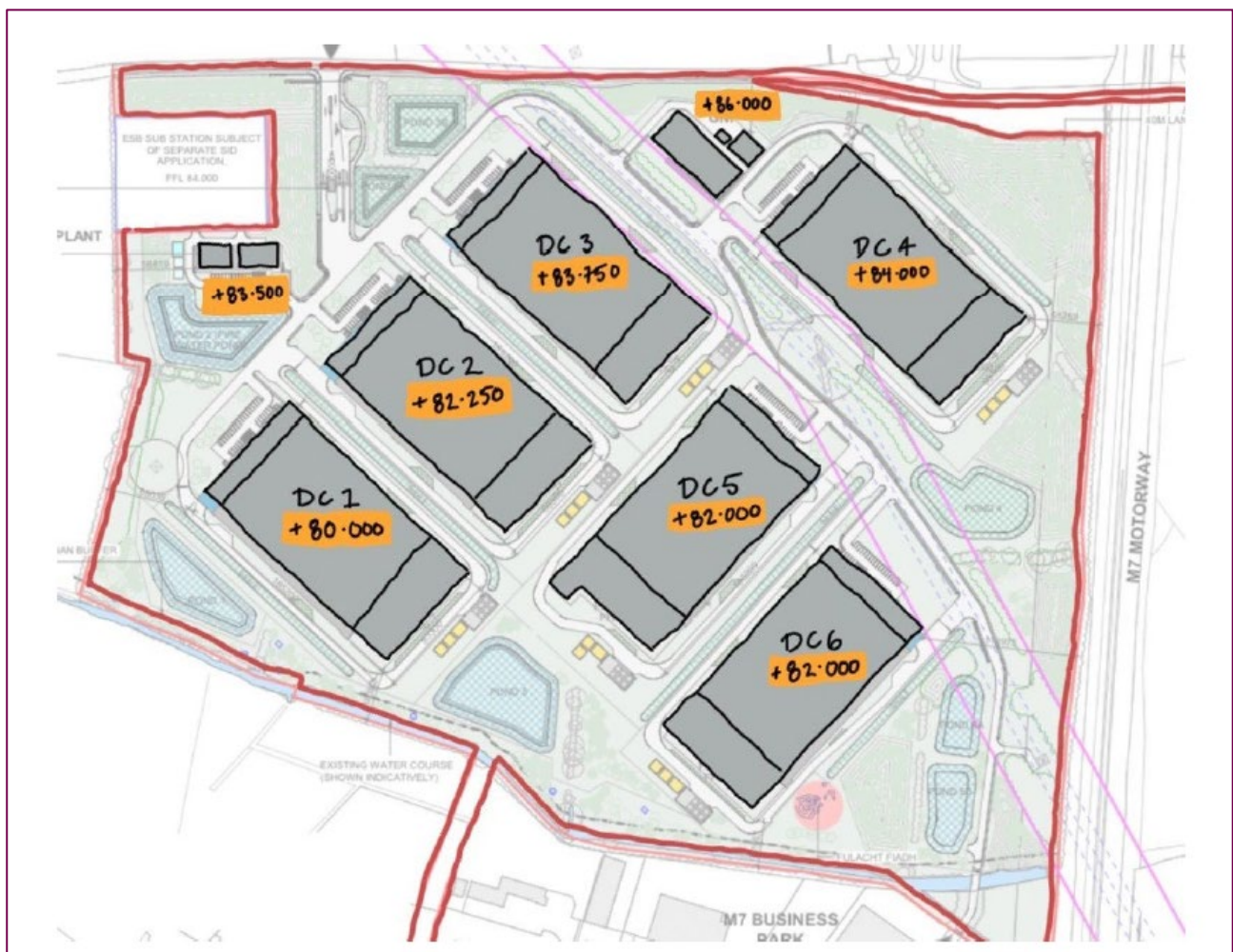
Figure 2.8: Sketch Site Plan with Proposed Levels (Data Centre Application - Architectural Design Statement, Volume II, Appendix 4.1)
